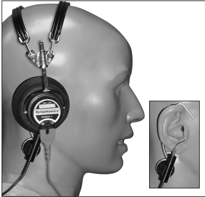
Figure 6.2.5A— Setup for the REDD measurement. The TDH earphone is placed on top of the probe mic setup.
